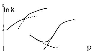
Fig. 7. The cases of competing mechanisms, and the resulting rate vs. pressure plots.
