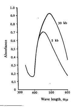
Fig. 1 Pressure spectra of 1,6-diphenyl-1,3,5hexatriene
