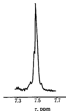
Fig. 12 NMR spectrum of PAN- \alpha d_1 at 100 Mc/sec in NaCNS- D_2O at 120°C
