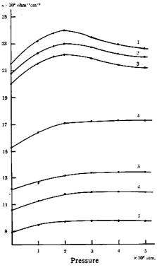
Fig. 3 Specific Conductivity of dodecyl trimethylammonium chloride at high pressure
