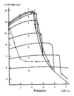
Fig. 2 Specific conductivity of dodecyl ammonium chloride at high pressure
