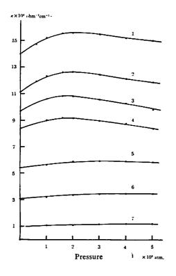
Fig. 4 Specific conductivity of dodecyl benzyldimethylammonium chloride at high pressure
