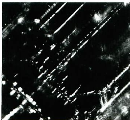
Fig. 7 The effect of electron irradiation on Laue patterns from LiF and NaCl crystals (a), as-grown LiF, 3.0 mm thick; (b) 1.5 \times 10^8 rad electron irradiated LiF, 7.6 mm thick; (c), as-grown NaCl, 3.0 mm thick; (d), 1.5 \times 10^8 rad electron irradiated NaCl, 5.8 mm thick.
