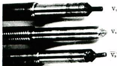
Photo. 3 Spindles of valves V_1 , V_2 and V_3 abraded by the detonations
