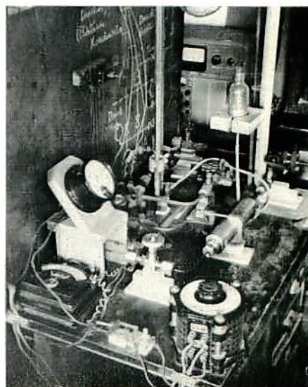
Apparatus for high pressure explosion, being manipulated at the right side of the steel wall protection— Laboratory of Physical Chemistry
