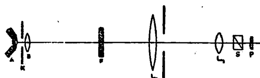
Fig. 1. Arrangement of the apparatus for illuminating the photographic plate by infra-red light.
